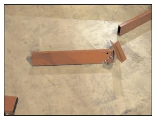
Insert Support Arm into Support Arm Bracket. Lock into place with two locking pins. Repeat for other Support Arm & Support Arm Bracket
