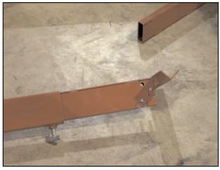
Insert assembled Support Arm Beam & Support Arm into Support Beam. Support Arm should be facing up with Locking Knob facing down for lifting Cabs & Bodies. Reverse for lifting truck beds
