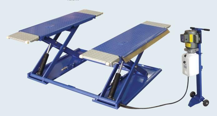
**S**PECIFICATIONS MR6K-38 6,000 lbs. Lifting capacity Overall width 76 1/2" Overall length 57 3/4" Track length 38" Maximum lifting height Collapsed height Motor 1 hp 110 vac Weight 1133 lbs.
