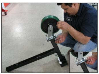
Install wheels onto four corner dolly supports with supplied bolts, lock washers & nuts. Tighten securely.
