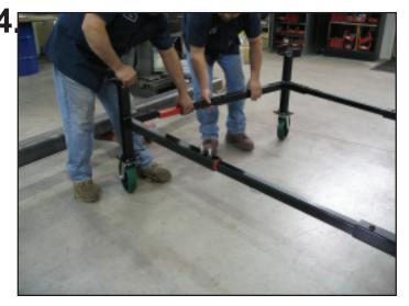
Continue attaching Extension Arms in this manner until you have the entire unit connected. Again, check to make sure all Frame Brackes are facing the same direction.
