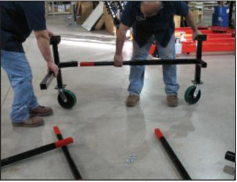
Connect it to the short arm of another Corner Support. The Frame Brackets on top of the Corner Brackets should be facing the same way.
