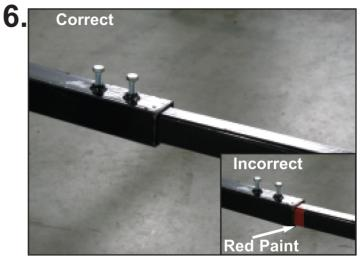
Adjust Dolly to desired width by sliding extension arms in or out and then securely tightening the locking bolts. For safety reasons NO RED PAINT should be showing on the Extension Arms. If red paint is visible then slide bracket into the the Corner support arm until it is no longer showing.
