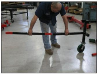
Insert Extension Arms into Corner Dolly Supports. Start by by installing the Extension Arm into the long arm of one of the Corner Supports.
