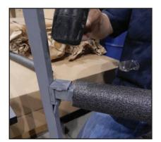
**3.** Repeat this step placing the tab of the short arm in the middle slot of the wall mounting bracket, and the remaining long arm in the bottom slot. Do these 3 steps with both wall brackets.
