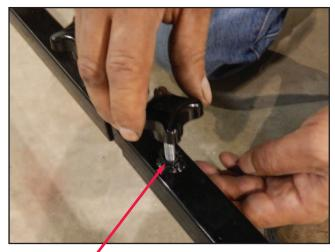
Secure the bottom support connector (D) and the bottom support beams (C) by screwing the supplied bolts into the welded nuts
