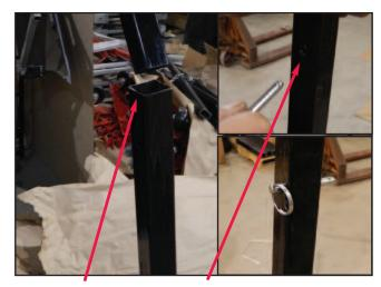
Slide the 48" upright (F) into the 46" upright (E). Align the holes of both uprights and insert locking pin (N). Do this step to both sides.
