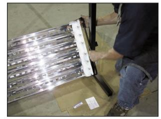
Place protruding 2" bolt (D) through provided hole in the bottom of upright Frame Structure (A). Place Hand Knob (E) on outside of Frame Structure (A) and tighten. Repeat on both sides.
