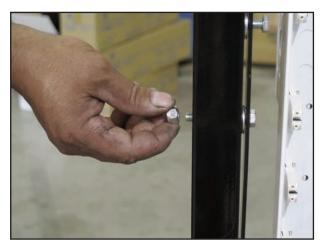
Repeat step 3 for middle Light Housing (C). NOTE: middle light will have 4 - 2" bolts (D) that will be tightened with Locking Nuts and will not be adjustable. Fully tighten nuts.
