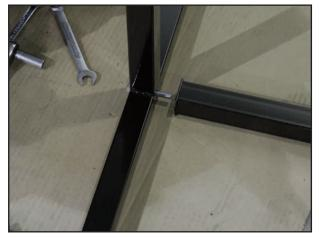
Attach straight bar of the Frame Structure (A) with 3" bolt (B)
