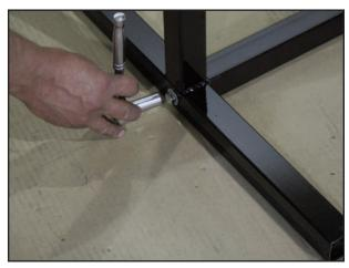
Fully tighten 3" bolt (B) to straight bar of the Frame Structure (A). Repeat step 1 and 2 for other side of Frame Structure (A) straight bar.
