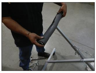
Place the foam pads onto the extension bars.
