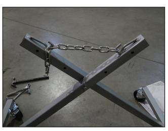
Attach the chain onto the hooks of each support base.
