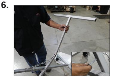
Insert the extension bar into the support base. Line up the holes and insert the pin. Place the 1" caps on either end of the bar. Repeat with the other extension bar.
